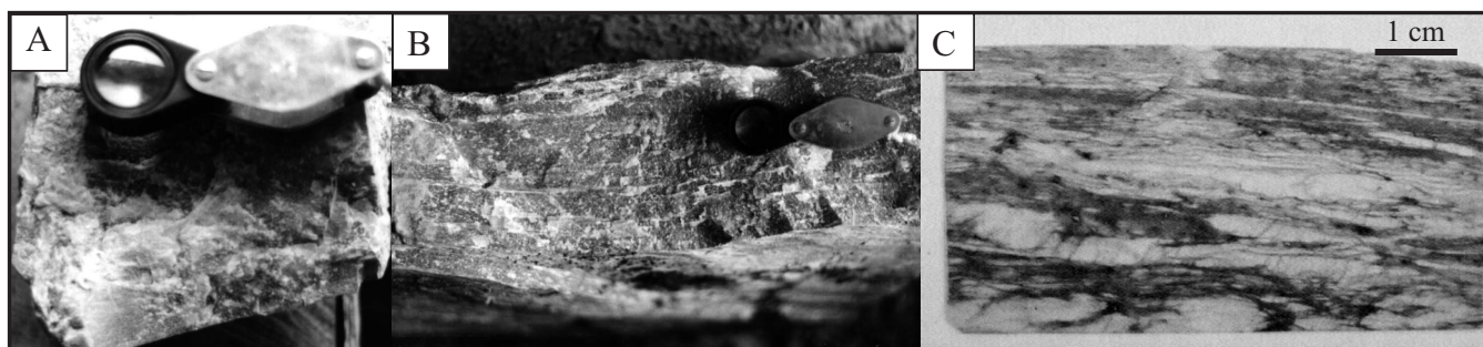
Fig. 10.- Photographs showing textural variation of the quartz vein at Limão. A) massive vein; B) laminated vein; C) laminated to schistose vein at the contact with the host rock.
