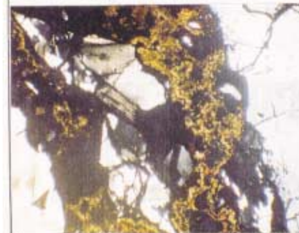
Figure 5.46c Photomicrograph of the mineralized quartz vein rich in jarosite (yellow) and iron oxide (hematite and goethite). Note the recrystallisation of the quartz vein. (XPL; TL; WOF = 2.5 \mu m; MG-R-229, Morro Pelado, São Francisco mine).
