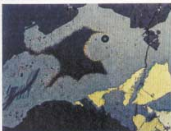
Figure 5.4a Hematite (gray-bluish tint) with pyrite, yellow colour. (PPL; RL; WOF = 400 \mu\text{m} ; MG-R-155, Itapetim District, Sertãozinho).
