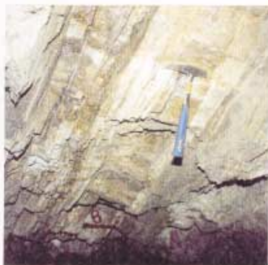
Figure 3.31 Mineralized quartz vein (syn-shearing) developed in mica schist concordant to the S 3 foliation (Shaft, Gurgueia area, Itapetim gold District, east domain; MG-R-165A).
