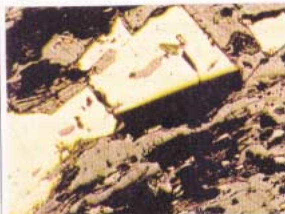
Figure 5.36 Recrystallisation product of pyrite (yellow; Type III) forming idiomorphic crystals. (PPL; RL; WOF = 750 \mu\text{m} ; MG-R-197; Igarape Garapa).
