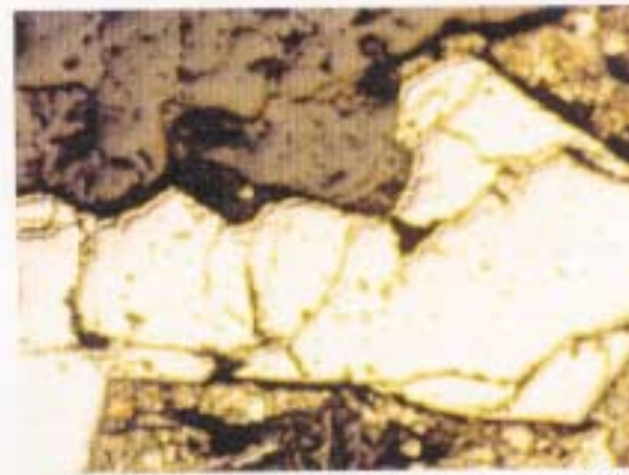
Figure 5.33 Deformation texture shows stylolitic indentation of porphyroblastic euhedral pyrite (Type II) due to pressure solution with a seam of pyrrhotite. (PPL; RL; WOF = 2500 \mu\text{m} ; MG-R-207; Santo Aleixo area).
