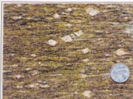
Figure 3.36a Augen gneiss (host rock for gold quartz veins) displaying intense mylonitic foliation (S 3 ) with flattened and symmetric porphyroclasts of K-feldspar oriented by shearing. (MG-R-205A, Santo Aleixo area, Guilhermina 'garimpo').
