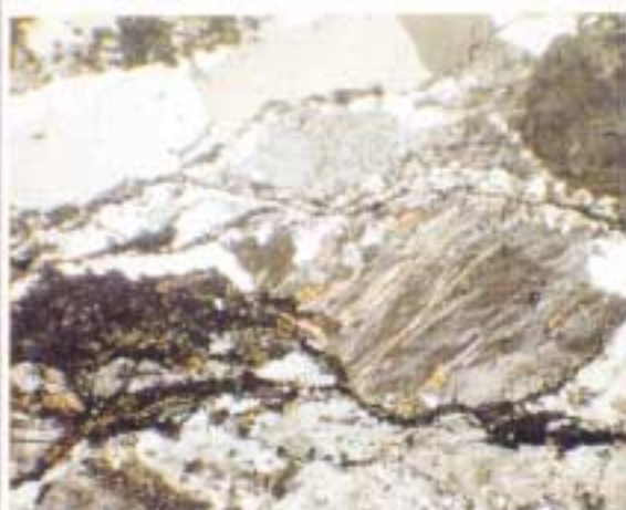
Figure 3.33 Gold-bearing quartz vein showing very intense degree of deformation. Recrystallisation has produced subgrains surrounding the margins of some grains, forming discrete bands of very fine quartz. Less recrystallised quartz ribbons occur showing annealed texture. These two quartz textures indicate that the degree of crystallisation is not constant. Note the needles of tourmaline included in the K-feldspar grains. Black areas (on the bottom left) are tourmaline fibres (XPL; TL; WOF = 3000 µm; MG-R-157B, Itapetim District, Sertãozinho).
