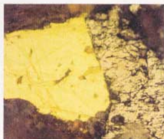
Figure 5.23 Coarse gold (bright golden yellow) associated with fractured pyrite (white-yellow) (PPL; RL; WOF = 1500 \mu\text{m} ; MG-R 197, Igarape Garapa).
