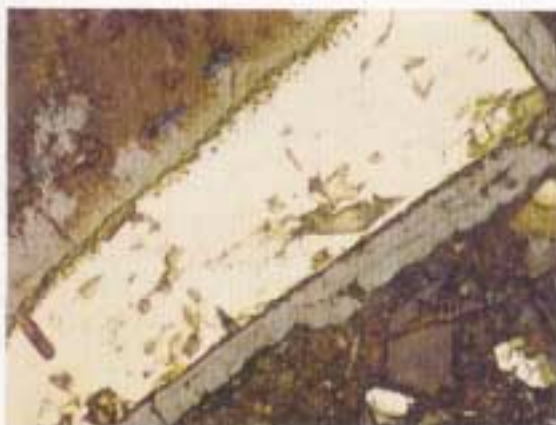
Figure 5.7 Photomicrograph of polished block showing pyrite (yellowish-white) crystal surrounded by hematite (grey) associated with small grains of covellite (blue) at the top left. (PPL; RL; WOF = 2500 \mu\text{m} ; MG-R-207, Santo Aleixo).
