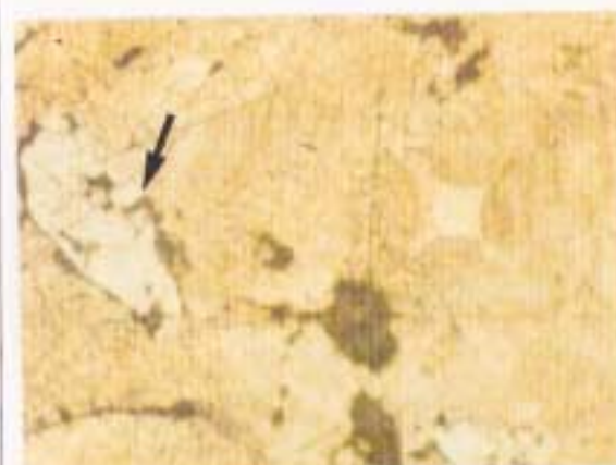
Figure 5.30 Zoned euhedral overgrowths of pyrite on cores of pyrrhotite (Type I). Cores of earliest formed pyrrhotite occur on the left (see the arrow; PPL; RL; WOF = 750 \mu\text{m} ; MG-R-229A; São Francisco mine).
