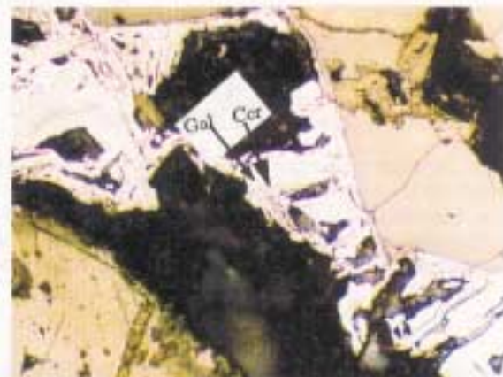
Figure 5.12 Polished block of galena (white) and cerussite (grey-white) forming zonal weathering texture. Black area is quartz gangue. (PPL; RL; WOF = 2500 \mu m; MG-T-111, Sertãozinho).
