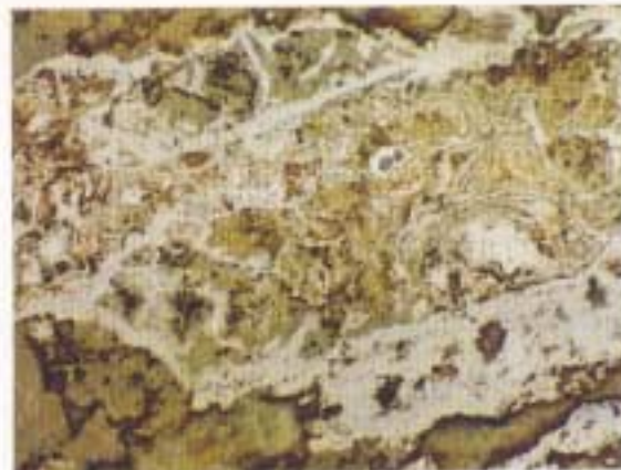
Figure 5.6 Photomicrograph of polished block showing hematite (white) rhythmically replaced by goethite (grey) during weathering. (PPL; RL; WOF = 750 \mu\text{m} ; MG-R-204I; Cmaffistula).
