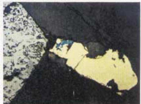
Figure 5.14 Chalcopyrite (yellow) replaced along fractures by covellite (blue), on the right side; on the left magnetite replaced by maghemite. (PPL; RL; WOF = 400 \mu m; MG-T-031, Sertãozinho, Itapetim District).
