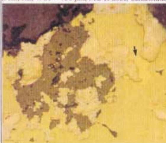
Figure 5.24 Coarse grain of gold (see the arrow) enclosed in coarse pyrite (white-yellow 'matrix') and associated with native bismuth (creamy tint). Uncharacterised selenium/tellurium minerals and bismuthinite are the very slight blue tinted areas; the dark area is quartz gangue. (PPL; RL; WOF = 750 \mu\text{m} ; MG-R-229C, São Francisco mine).
