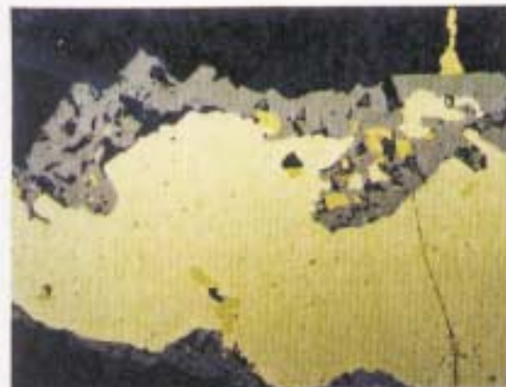
Figure 5.5 Pyrite (yellowish-white) surrounded by hematite (gray-bluish). Chalcopyrite (brassy-yellow) occurs as inclusions in both minerals (PPL; RL; WOF = 400 \mu\text{m} ; MG-T-034, Pimenteiras).
