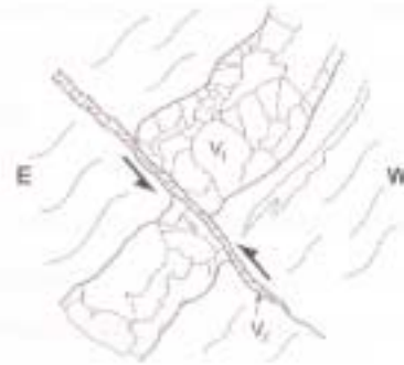
Figure 3.41b Sketch of Fig. 3.41a illustrating the concordant gold mineralized quartz vein ( V_1 ; S 60^{\circ} E ) banded when cross-cut by the discordant vein ( V_2 ; N40^{\circ} E ) indicating a sinistral sense of movement (Boqueirão dos Cochos area; MG-R-208B).
