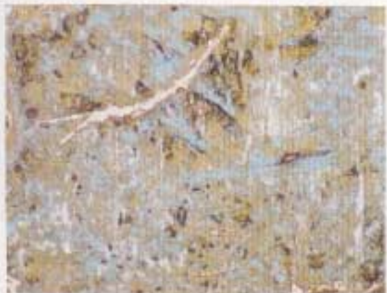
Figure 5.13 Disintegration of chalcopyrite (yellow-brownish) to a network of covellite (blue). Note the incipient decomposition of covellite to chalcocite (white lamellae). (PPL; RL; WOF = 400 \mu m; MG-R-210, Santo Aleixo).
