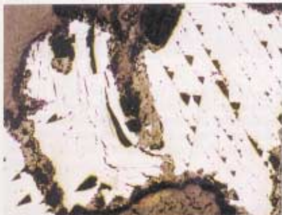
Figure 5.11 Photomicrograph of polished block of galena (white); cleavage pits do not show any evidence of deformation (PPL; RL; WOF = 1500 \mu m; MG-R-197, Igarape Garapa).
