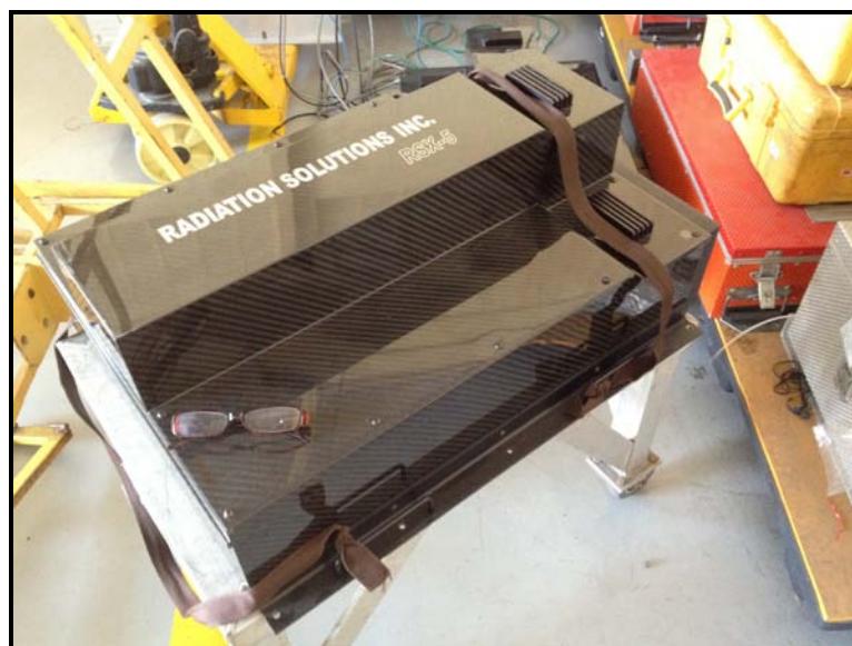
Figura 5 – Gamaespectrômetro Radiation Solution RS-500.
