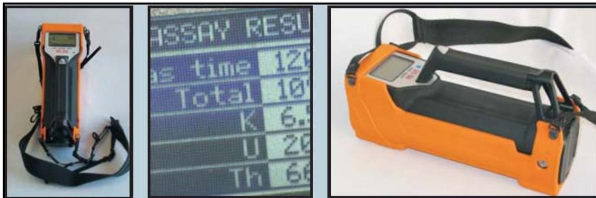
Figura 2 – Gamaespectrômetro Portátil RadiationSolutions RS-230 Super-SPEC.
