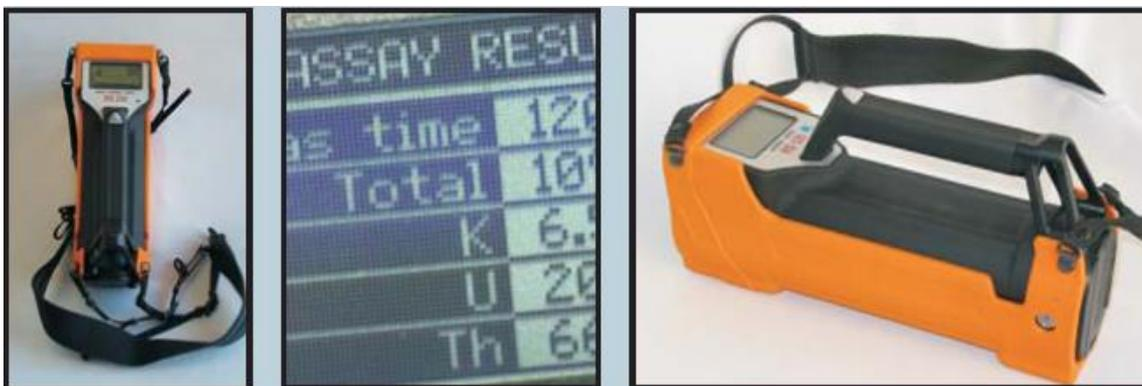
Figura 1 – Gamaespectrômetro Portátil Radiation Solutions RS-230 BGO SUPER SPEC.
