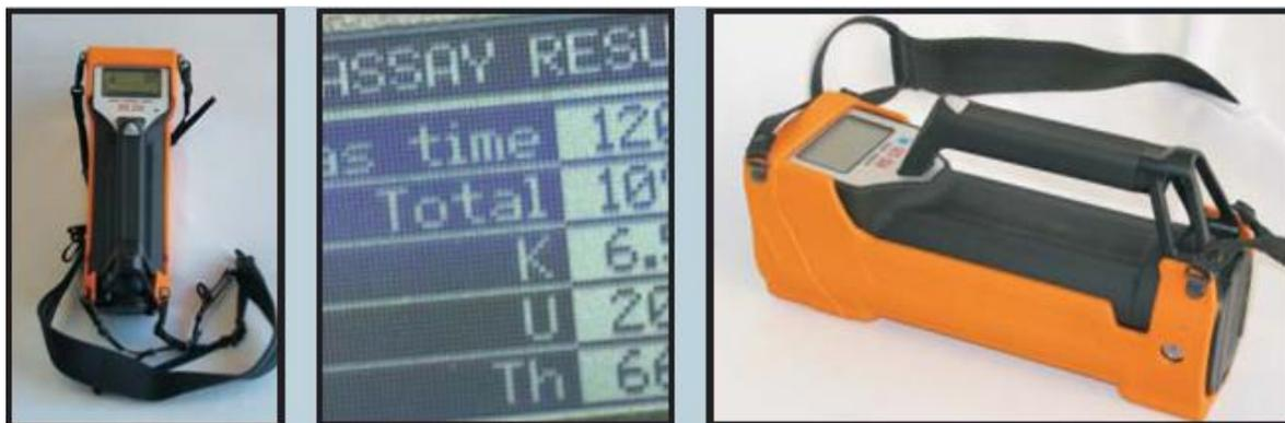
Figura 1 – Gama espectrômetro Portátil Radiation Solutions RS-230 Super-SPEC.
