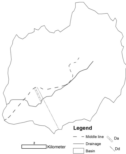
Fig. 3. An example of TecDEM in obtaining the T-Factor. Da = Distance from the basin bisector to the current drainage. Dd = Distance from the basin bisector to the border of the basin. Distances are measured perpendicular to the trunk drainage channel.
