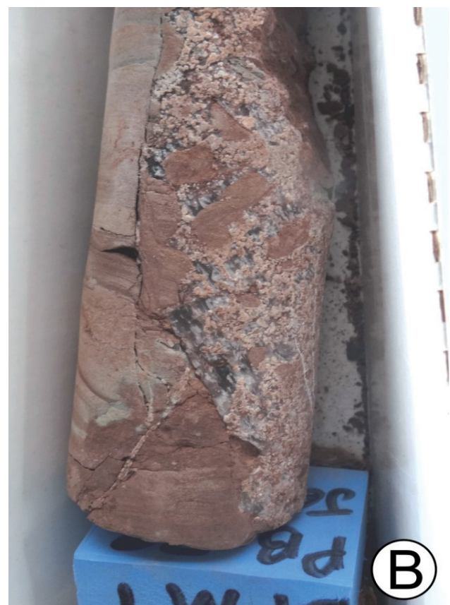
Figure 4: Drill hole PB-01-RO cores: phosphate-bearing calciferous rhythmite evidencing diagenetic alteration: A) veining (cm-scale); B) brecciation (core width = 5 cm).
