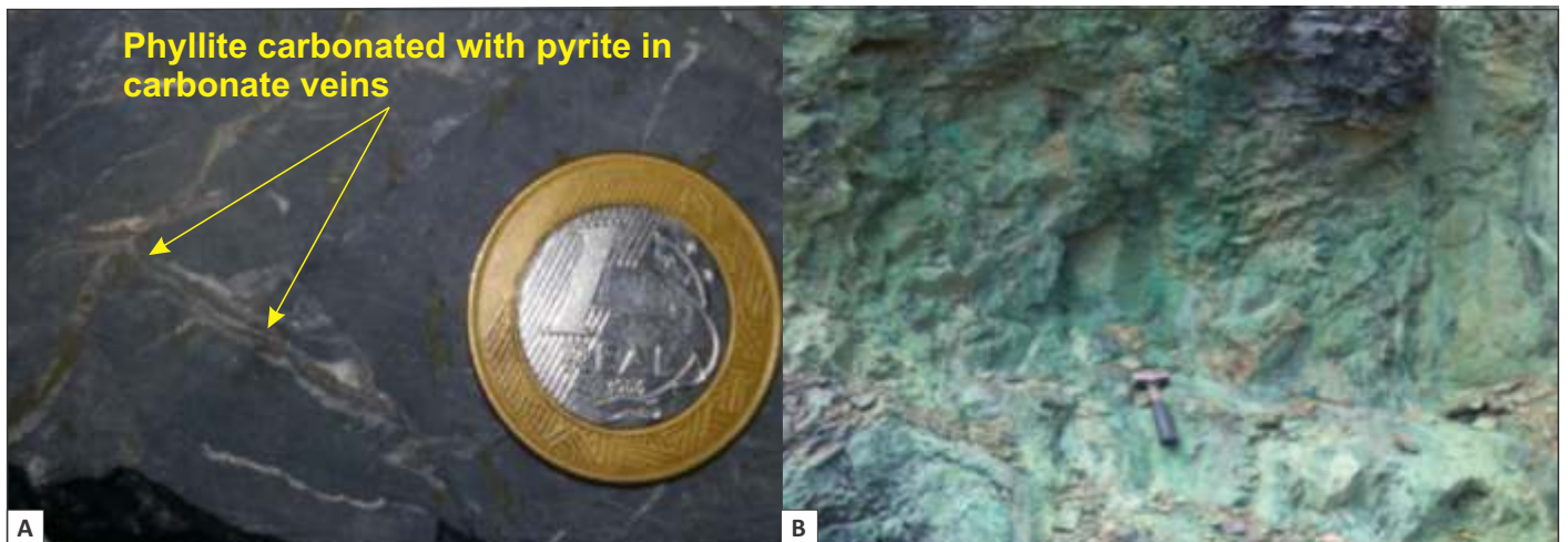
Figure 07 - Hand specimen and rock exposure from Pedra Verde mine: (A) Borehole sample of phyllite carbonate with sulfide-rich carbonate veins. (B) Malachite resulting from leaching of phyllite carbonate.
