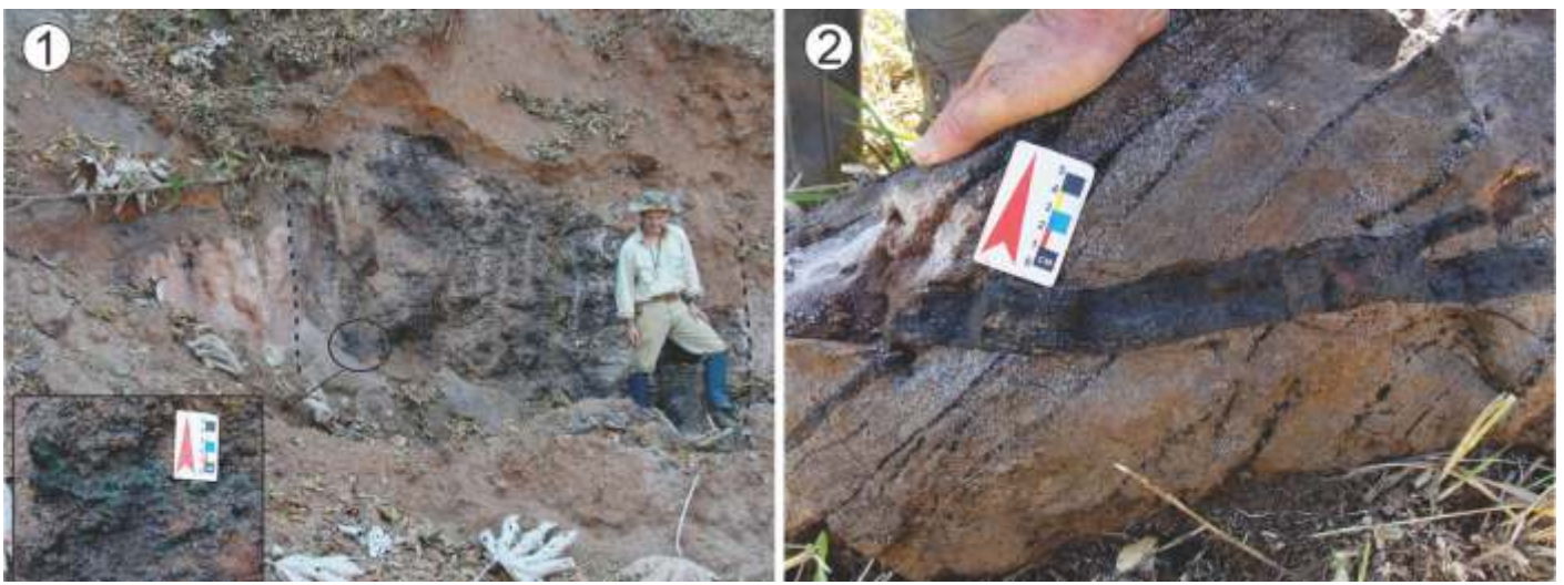
Figure 06 - (A) Gossan exposure including a massive sulfide vein (4 m thick) hosted by paragneiss of the Migrantinópolis Formation. Sample from this outcrop contains quartz, sulfides, gahnite and iron oxides, with composition of 5.9% Zn, 0.74% Pb and 0.17% Cu; (B) Hand specimen showing weathered sulfides along the foliation plane and in veins, with composition of 0.61% Zn, 1.1% Pb and 0.24% Cu.
