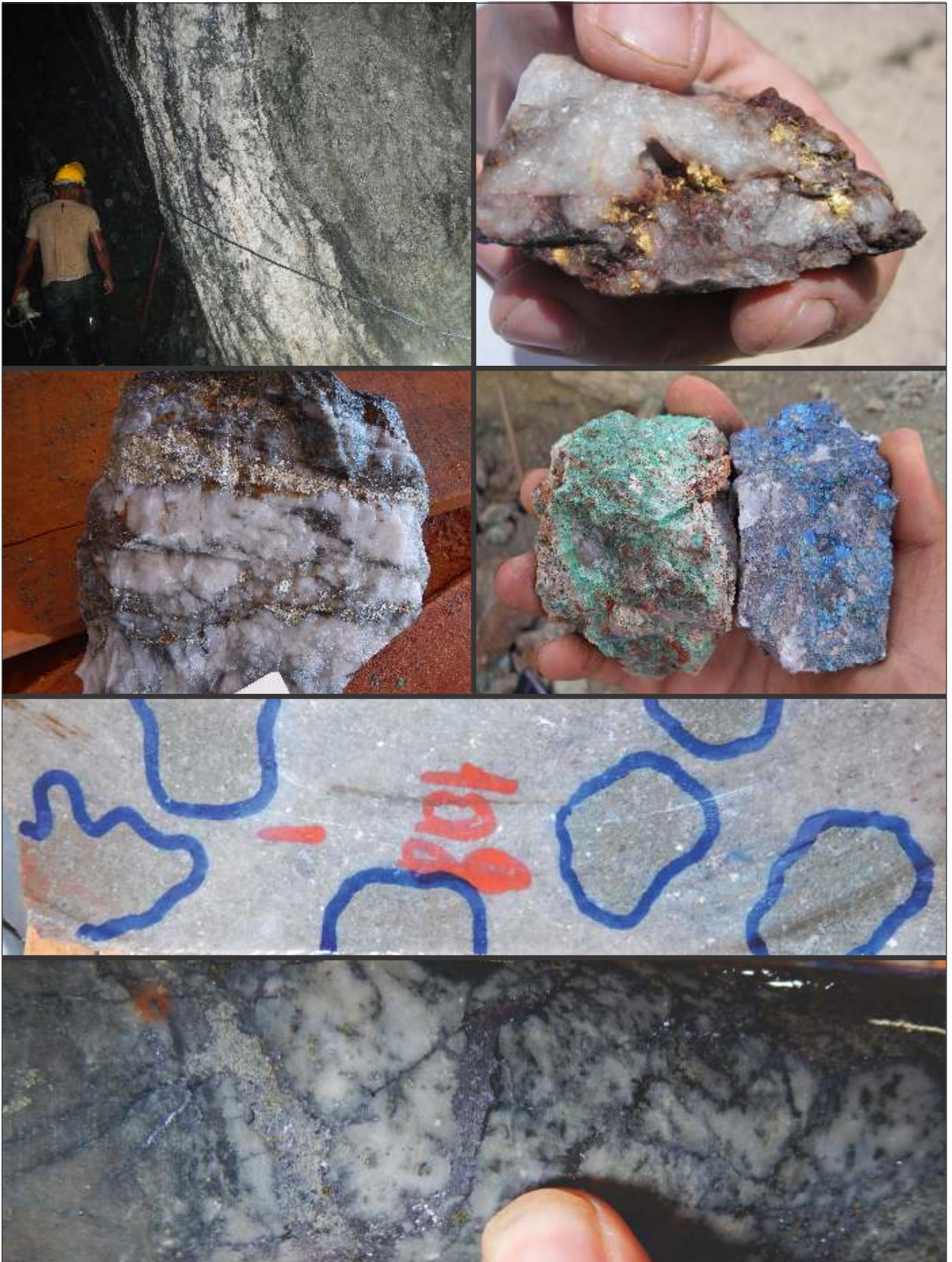
Figure 06 - Exposure and hand specimen from the Peixoto de Azevedo gold district. (A) Banded quartz vein with quartz bands alternating with chlorite and sulfides bands, as exposed at Serrinha do Gurantã gold deposit shaft. (B) Free gold in rusty sulfide-rich quartz vein from Valentim deposit. (C) Quartz vein with chlorite and pyrite bands. (D) Vein samples from Serrinha do Gurantã deposit with copper-rich sulfides (bornite and chalcocite) and secondary copper minerals (malachite, azurite and chrysocolla). (E) Cut sample of granite from X1 deposit with phyllic alteration and disseminated pyrite (blue circles). (F) Hand specimen of hydrothermal breccia from Gurantã Ridge deposit, with venules filled by galena and disseminated chalcopyrite.
