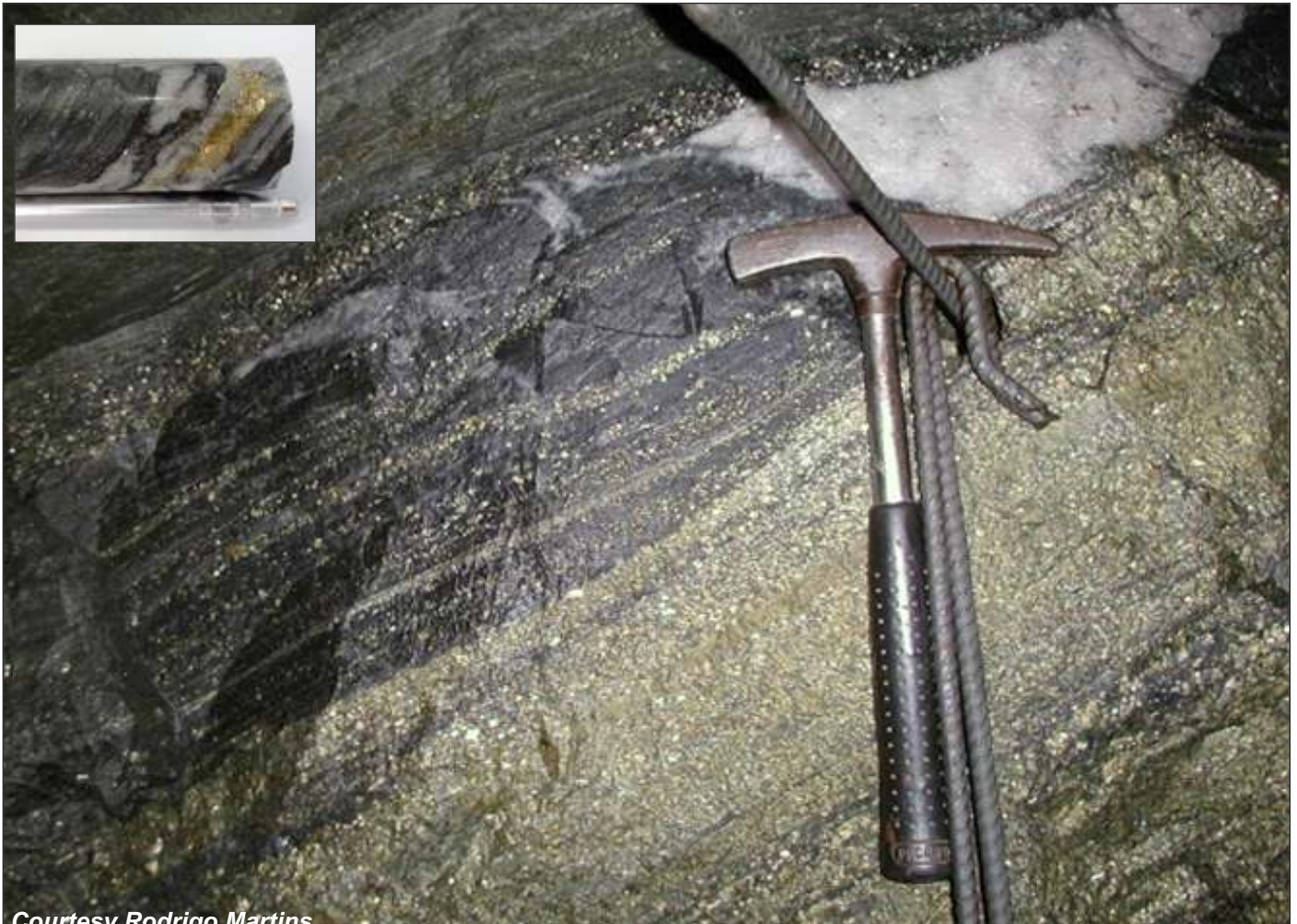
Figure 09 - Rock exposure of banded and massive sulfide ores. Insert photo of a drill core section presenting free gold in a quartz vein (Cuiabá mine).
