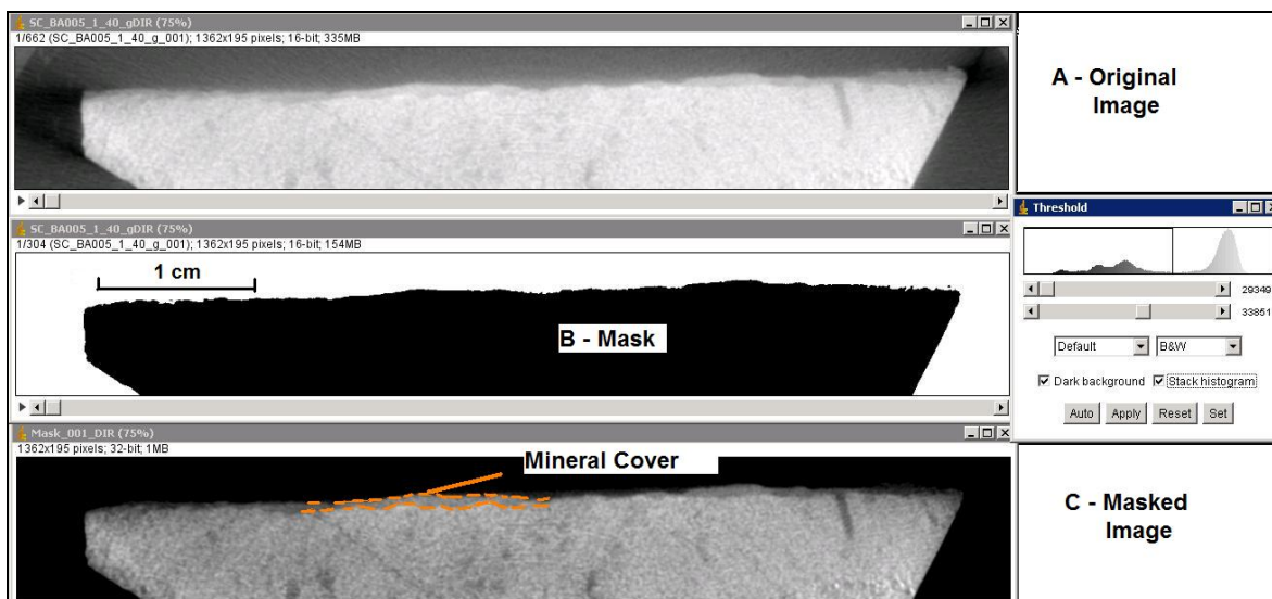
Figure 4. Application of a threshold to isolate the sample 1 from surrounding air. (A) Original image. (B) Histogram and mask image. (C) Masked image - outside as NaN (Not a Number).
