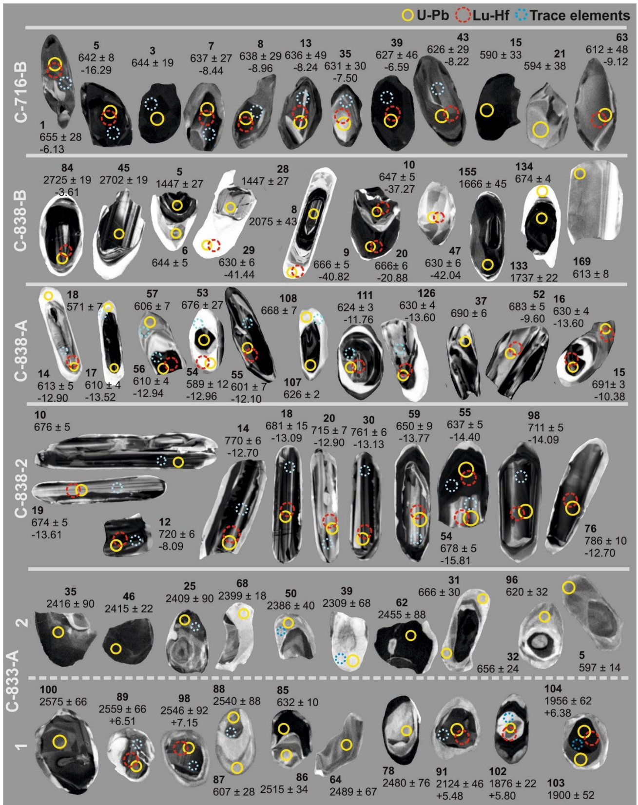
Figure 3.6: Cathodoluminescence (CL) images of representative zircon grains. Location of the spot analyses and corresponding ^{206}\text{Pb}/^{238}\text{U} or ^{207}\text{Pb}/^{206}\text{Pb} dates in Ma marked with yellow circles (spot size ~30 microns), blue dashed circles for trace elements (spot size ~20 microns), and dashed red circles for Lu-Hf (spot size ~50 microns).
