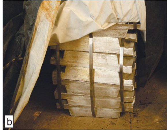
Fig. 4.5: a) Alloy with Sn grades between 10 to 15%. This product is sold for its high Pb content, making the Sn just a by-product, b) Ingots of high quality Sn that match the LME standard.
