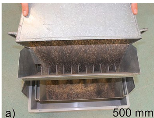
Fig. 6.8: Sample splitting with riffle splitter: a) 500 mm splitter for samples up to 100 kg, b) 180 mm splitter for samples up to 2 kg.
