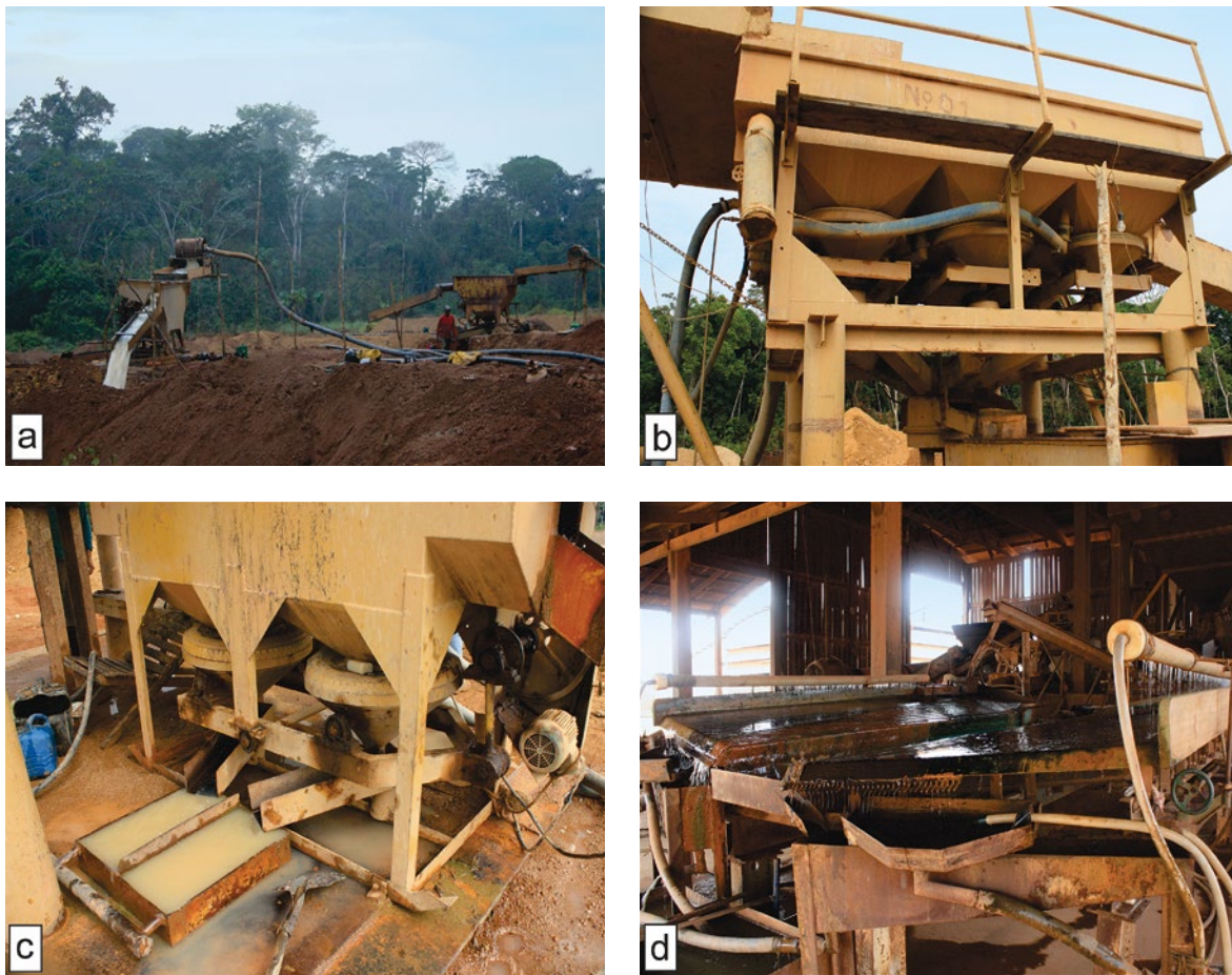
Fig. 4.2: a) Jigs outputting clay as tailings in the first gravity concentration, b) and c) Jigs separating the cassiterite and the first and second cama (basin under the jig), d) Shaking table separating the very fine cassiterite.
