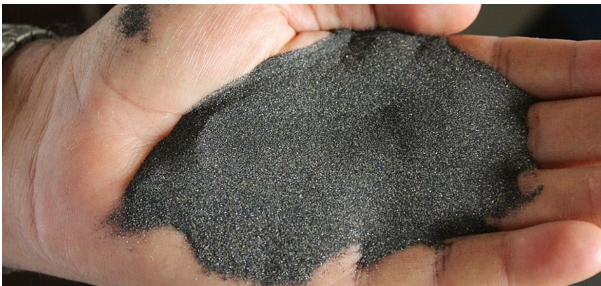
Fig. 4.4: Final cassiterite concentrate product after magnetic separation at the CEMAL plant.
