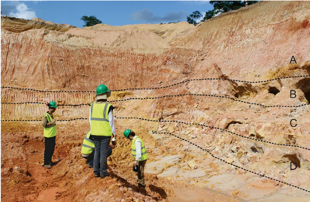
Fig. 3.10: Mining site in the Santa Bárbara deposit, where an overburden of massive mottled clay covers mineralized sand layers.
