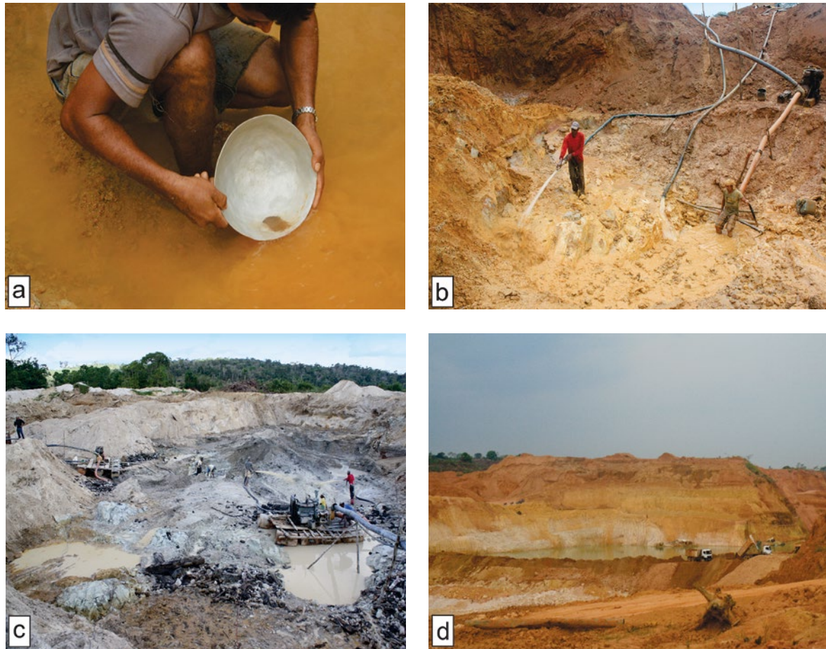
Fig. 4.1: a) Garimpeiros checking if the layer contains enough cassiterite to be mined, b) Mining operation with an hydraulic jet in Massangana, c) Mining of alluvium near the Massangana River, in Garimpo Massangana, d) Use of heavy machines to mine in Garimpo Bom Futuro.
