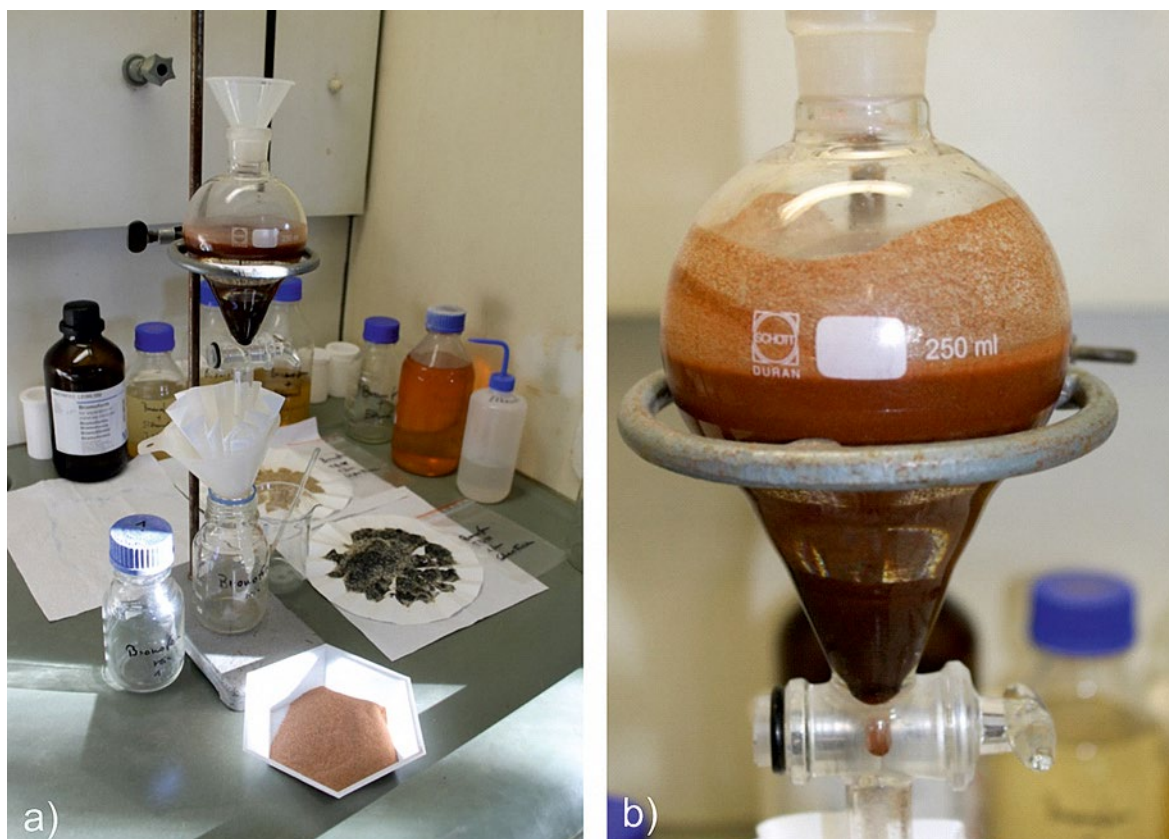
Fig. 6.9: a) Laboratory equipment for heavy liquid separation, b) Funnel with 200 ml \text{CHBr}_3 and stirrer.
