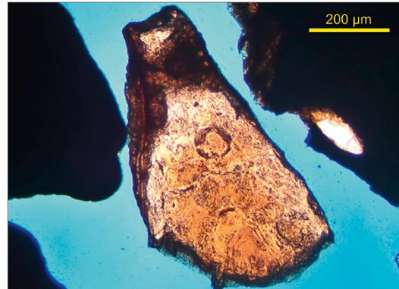
Fig. 10.20A: Section #06, RM, 125x, ||: Isolated euxenite grain with pyrochlore alterations (darker zones).
