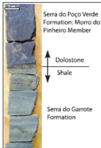
Fig. 7. The sharp contact between shales of the Serra do Garrote Formation and dolostones of the Morro do Pinheiro Member (Serra do Poço Verde Formation). Note the thin layer of sulfides exactly at the contact.
