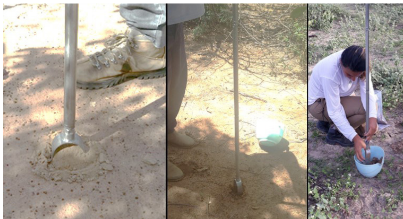
FIGURE 9 - Auger drilling sampling. Picture by Aline Nogueira.
