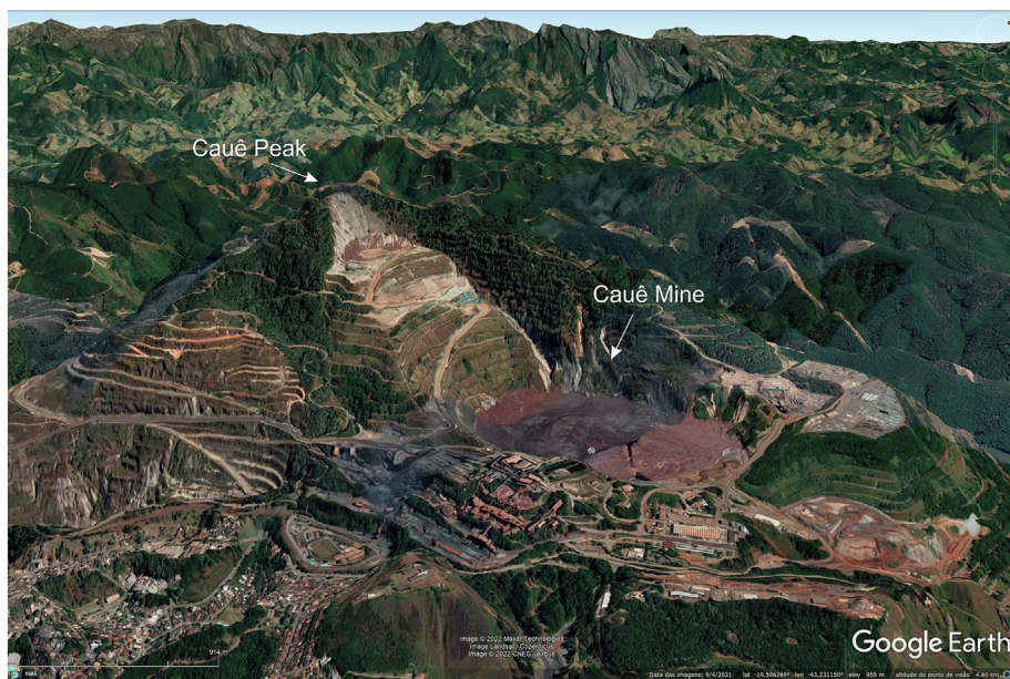
Fig. 5. Google Earth satellite image from Cauê Peak today. The open pit is being filled with tailings. Source: Google Earth in 2022.
