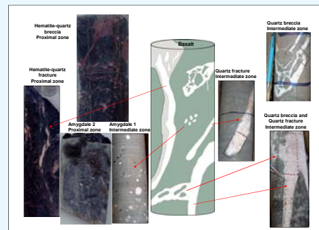
Fig. 3 – Schematic diagram showing classification and timing relationships of the veins.
