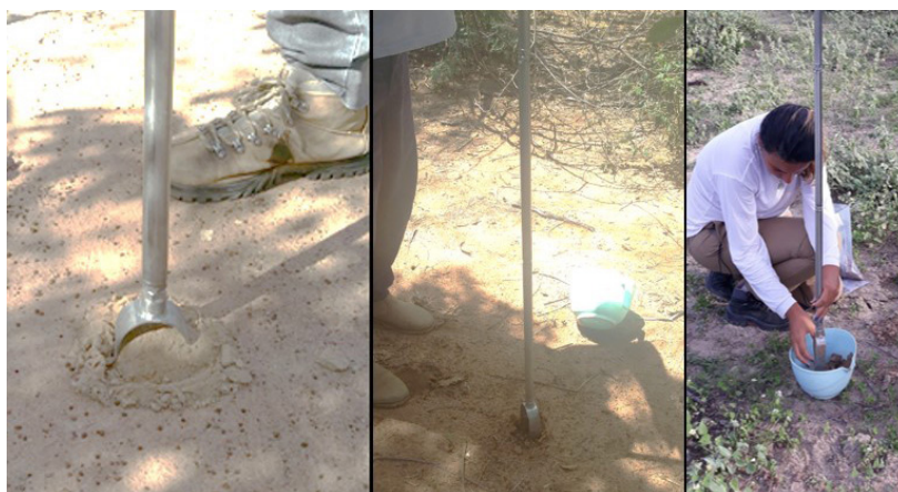
FIGURE 9 - Auger drilling sampling. Picture by Aline Nogueira.
